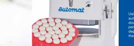
Using the Fortuna semiautomatic machines, the dough pieces become perfectly high and round. The deposition is performed with the end downwards.
