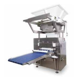
The flexible 4- to 6 pocket Primus Pro, covers made of stainless steel, can be operated comfortably and meets the latest hygiene requirements as a result of the separation of drive and dough area. The individual assemblies, such as the pre-divider or the pressing piston can be easily dismounted and cleaned.
